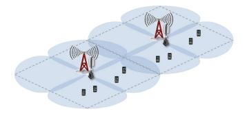
Co-locate A8n with existing 3G/LTE cell site to offload traffic for an almost identical cell area.
